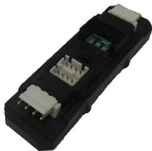
Figure-8c: KXCBA CANBus terminal
